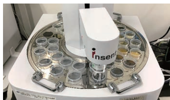
▲味認識装置を用いた食肉の呈味性の評価 Evaluation of meat flavor using a taste sensing system
