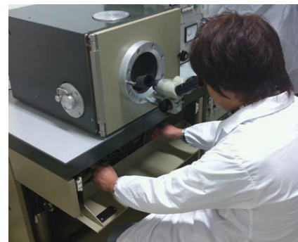
▲凍結切断・レプリカ標識法を用いた生体膜分子の微細局在分布の解析 Nanoscale analysis of biomembrane molecular distribution using the freeze-fracture replica labeling method
