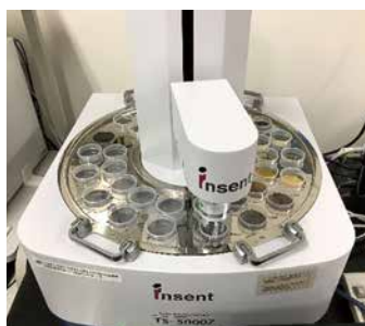
▲味認識装置を用いた食肉の呈味性の評価 Evaluation of meat flavor using a taste sensing system
