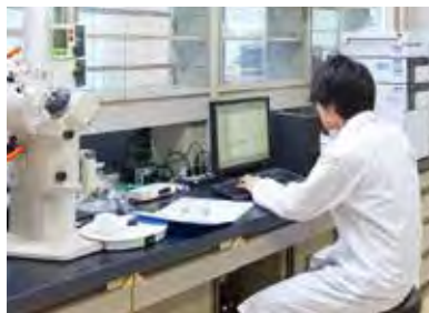
◀UPLCを用いたホモシステインの定量 Homocysteine determination using an ultra performance liquid chromatography (UPLC) system
